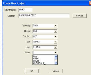
Fill in the New Project name, Location and use the dropdown window in each of the cells to select which shapefile attributes are to be used to create the stand masters. This process forces the user to create the stand masters in a new FLIPS project in order to safeguard the existing FLIPS data. You can then use Stand Maintenance in FLIPS to copy the new masters from one FLIPS project to another.
