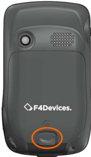
2. If your model has the 3.5G connection function, you need to install the SIM card provided by your mobile operator and insert the card all the way into the slot then push to lock.
