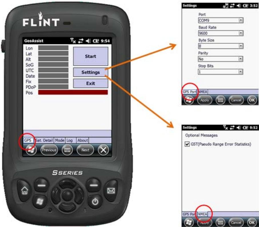
GeoAssist will access COM 9 and, once locked onto satellites, display the GPS data.
