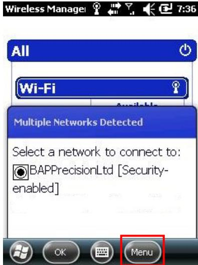
3. If more than one network is detected, the screen will display a network list. Tap the desired network and follow the procedure to configure the wireless network.
